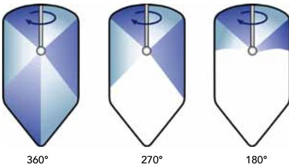
Depending on the type of DUNOS<sub>R</sub>, a different jet image is produced on the vessel surface.
