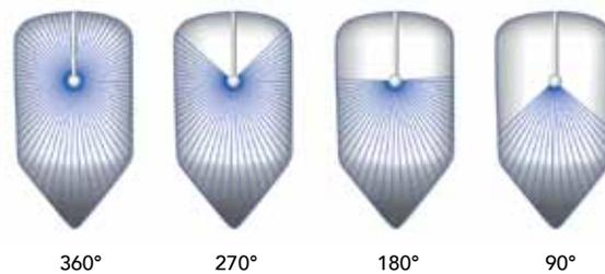
Depending on the type of DUNOS<sub>s</sub>, a different jet image is produced on the vessel surface.
