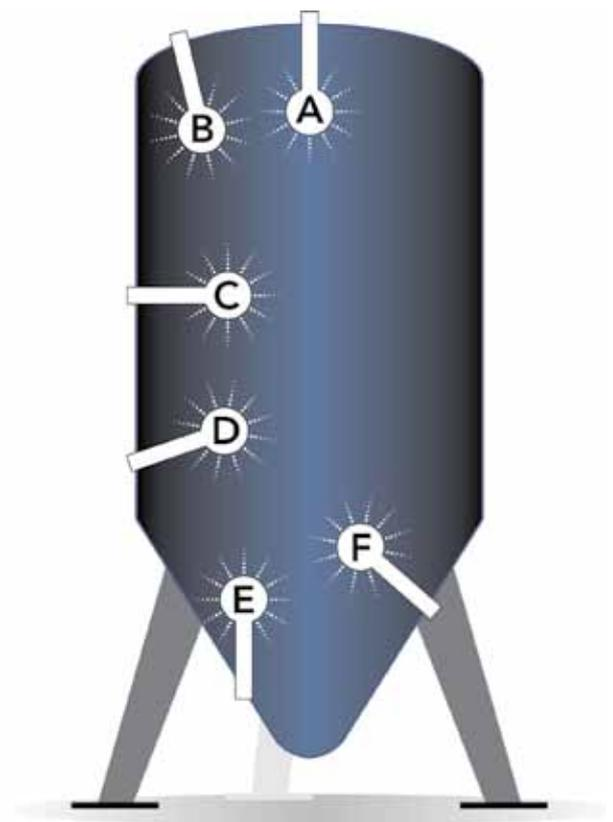
KIESELMANN spray heads can be fitted in every position into your tank.
