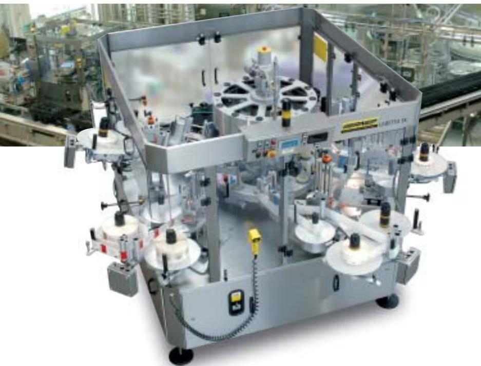
**Fully-automatic labelling machine for containers made of glass, plastic, metal, and moulded containers.**
